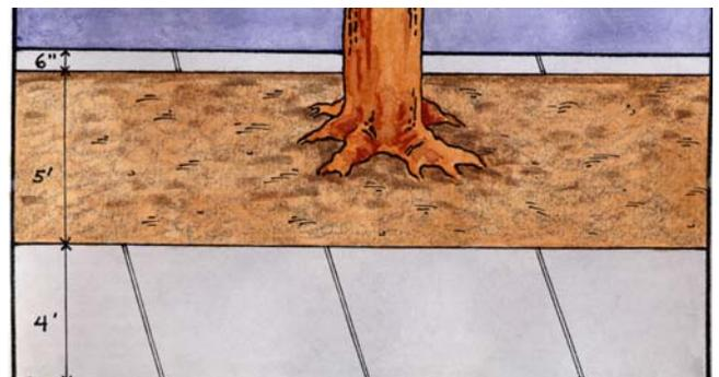
Tree pits can be expanded by removing excess concrete to form a planting strip to allow tree roots space to grow and reduce the chance of a lifted sidewalk. It also allows rain to permeate the ground.
