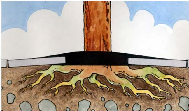
In severe cases, the cement block can be removed and filled with patch cement or blacktop. The borough prefers Sactrete or patch cement to blacktop.
